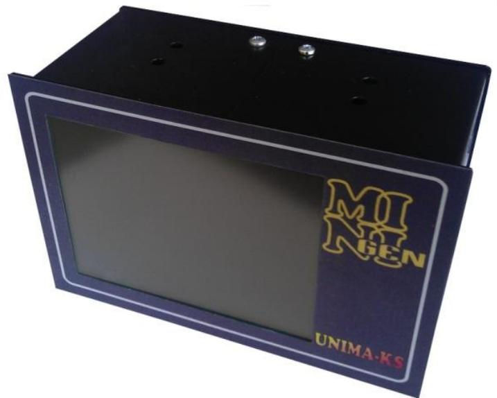
**Control system for cogeneration units and other engine-generator sets with a color graphical LCD 320x240 points display with touch-screen, wide range of management, communication and configurability. Supports all modes of operation with the grid, manual, semi automatic or automatic mode, control of energy output and input from the mains, power sharing between multiple units (virtual concentrator), etc.**
